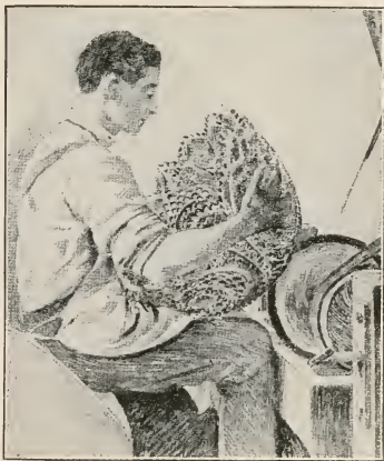
Polishing a large cut-glass bowl on a wooden wheel
